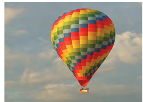
Heated air inside a hot air balloon causes the balloon to rise due to convection.
